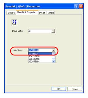
• The maximum value of the RAM Disk area is 67108864. When the value over the maximum value is set, an error occurs.
